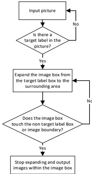
Fig. 3: Edge extension clipping method
