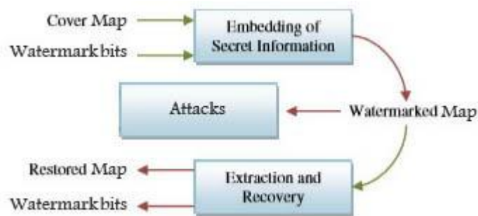
Fig. 1: Basic reversible map watermarking scheme.
