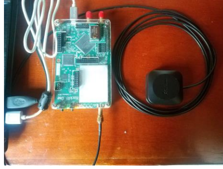
Fig. 2: HackRF one and the microstrip antenna.
