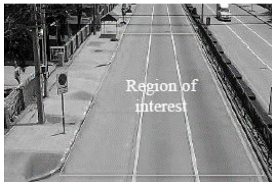
Fig. 3: Region of Interest (ROI) in a vehicle counting system.
