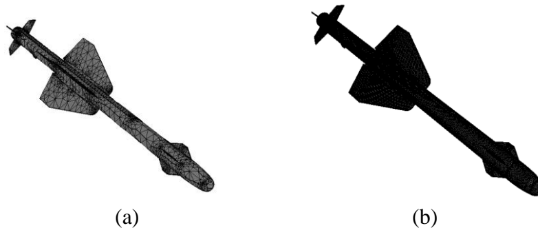
Fig. 3. Polygonal models of a missile generated Creo (a – number of triangles is 12000, b – number of triangles is 143000)
