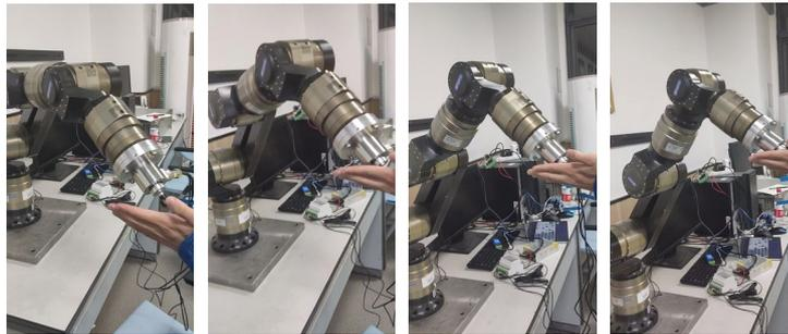
Fig. 5: Compliant dragging process of robot.
