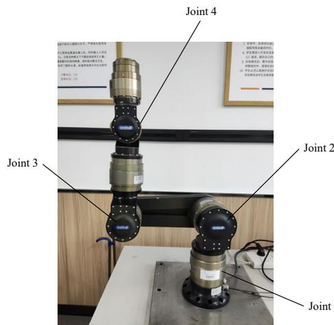
Fig. 1: Structure of SCHUNK robot.
