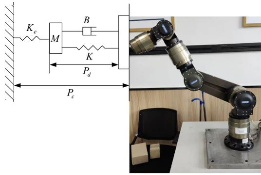
Fig. 4: Contact model between robot and environment.
