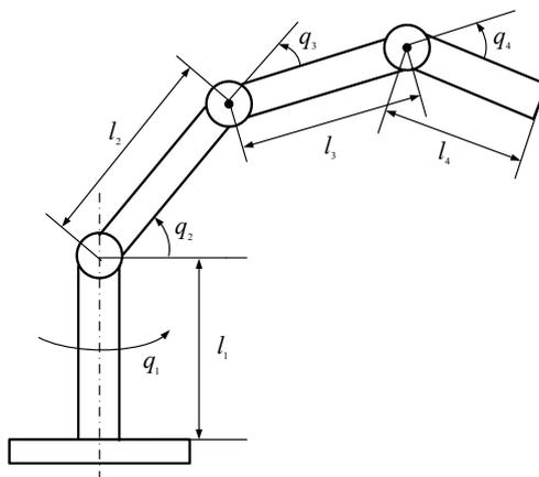
Fig. 2: Mechanism diagram of the robot.
