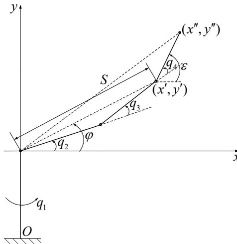
Fig. 3: Coordinate diagram of the mechanism.
