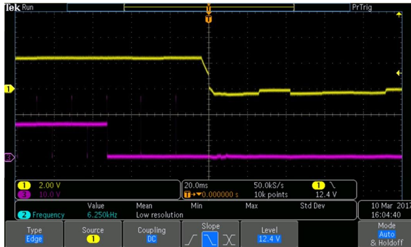
Fig. 11: Test Result of Hardware Fault Insertion
