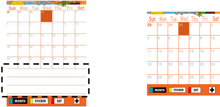
(a) 768×1280, 320 DPI. Correctly displayed. (b) 480×800, 240 DPI. The bottom note disappears.
