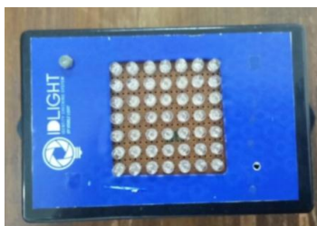
Fig. 2: LED beacon controlled by Arduino Nano.
