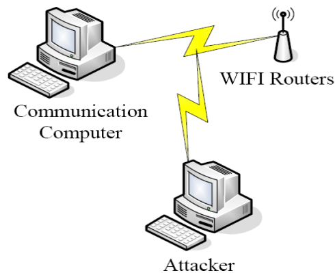
Fig. 1: Topology graph of testing attacks on WEP.
