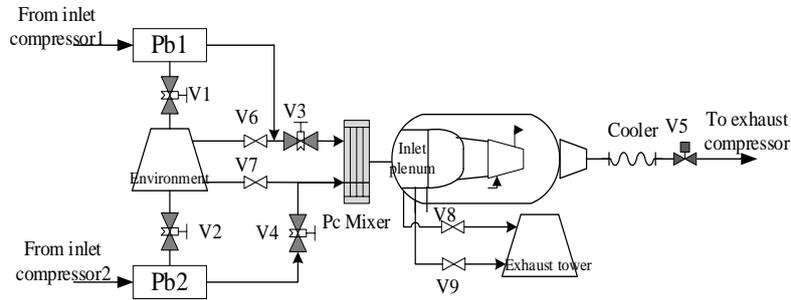
Fig. 2: Schematic diagram of ATF flight environment simulation system
