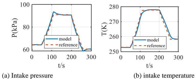
Fig. 4: Intake pressure and intake temperature control effect
