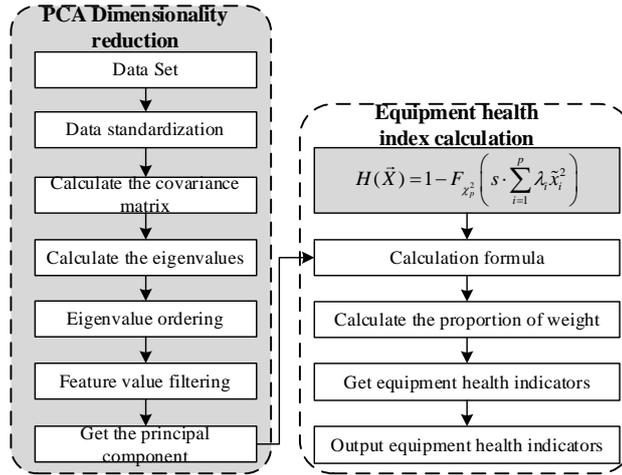
Fig. 1: PCA-SPR-based performance evaluation process
