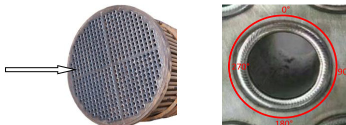
Fig. 1: all-position welding of tube-sheet
