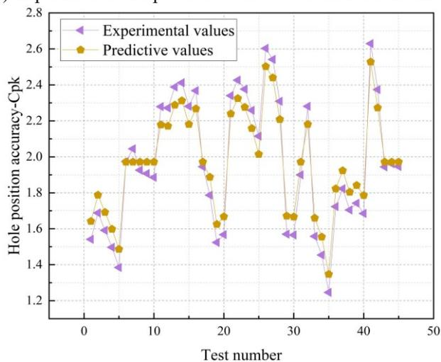
(c) Effect of hole quantity, feed rate and spindle rotation speed on hole position accuracy
