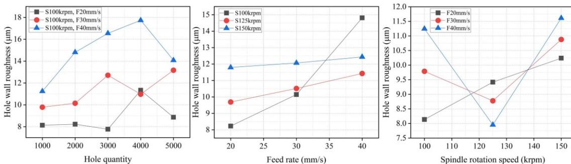
(a) Effect of hole quantity, feed rate and spindle rotation speed on hole wall roughness
