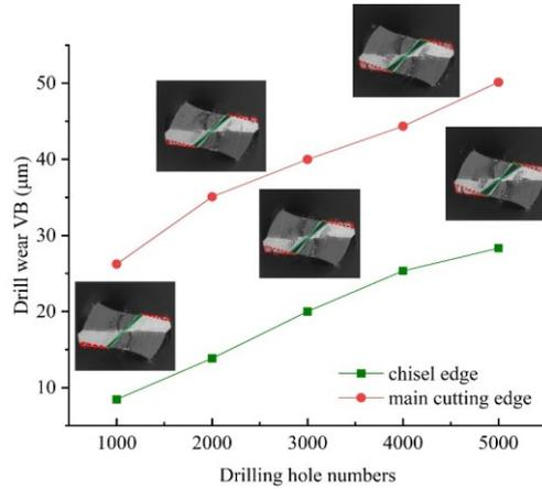
Fig. 3: The relationship between the hole-drilling number and drill wear.
