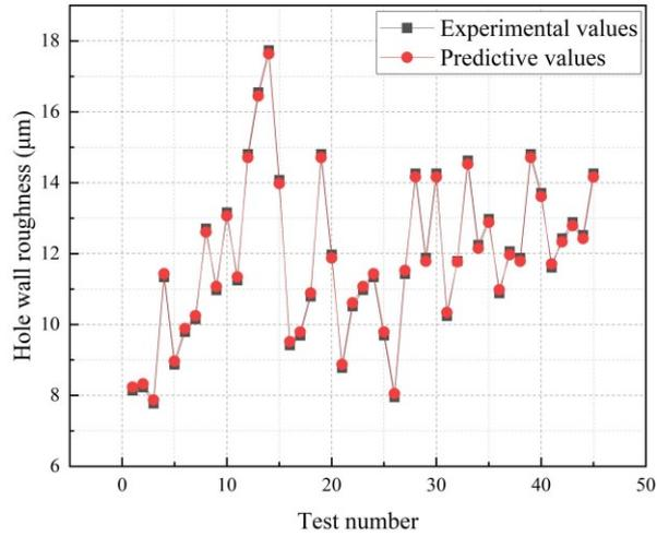
(a) Experimental and predictive values of hole wall roughness
