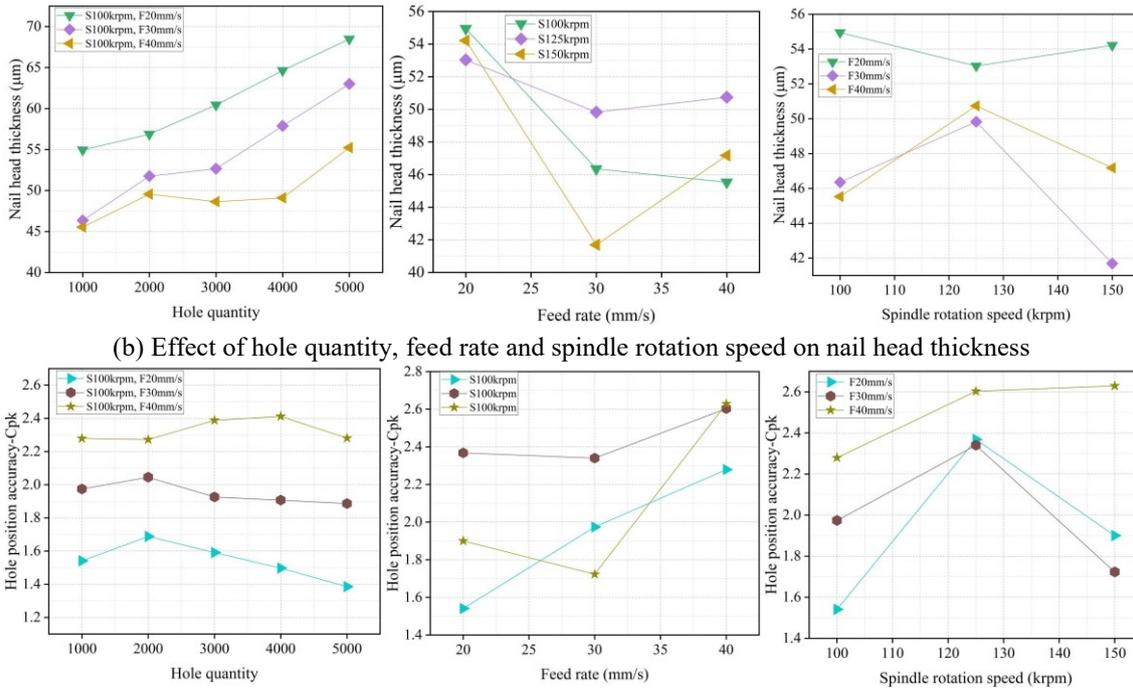
(c) Effect of hole quantity, feed rate and spindle rotation speed on hole position accuracy
