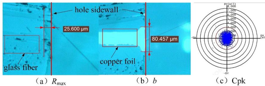
Fig. 4: The hole-drilling quality.
