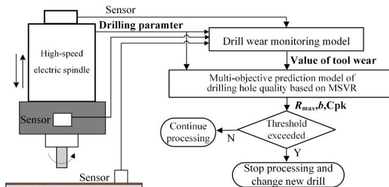
Fig. 1: Diagram of hole quality control for multilayer PCB.
