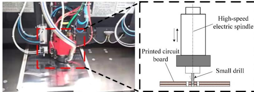
Fig. 2: High-speed drilling experiment setup.
